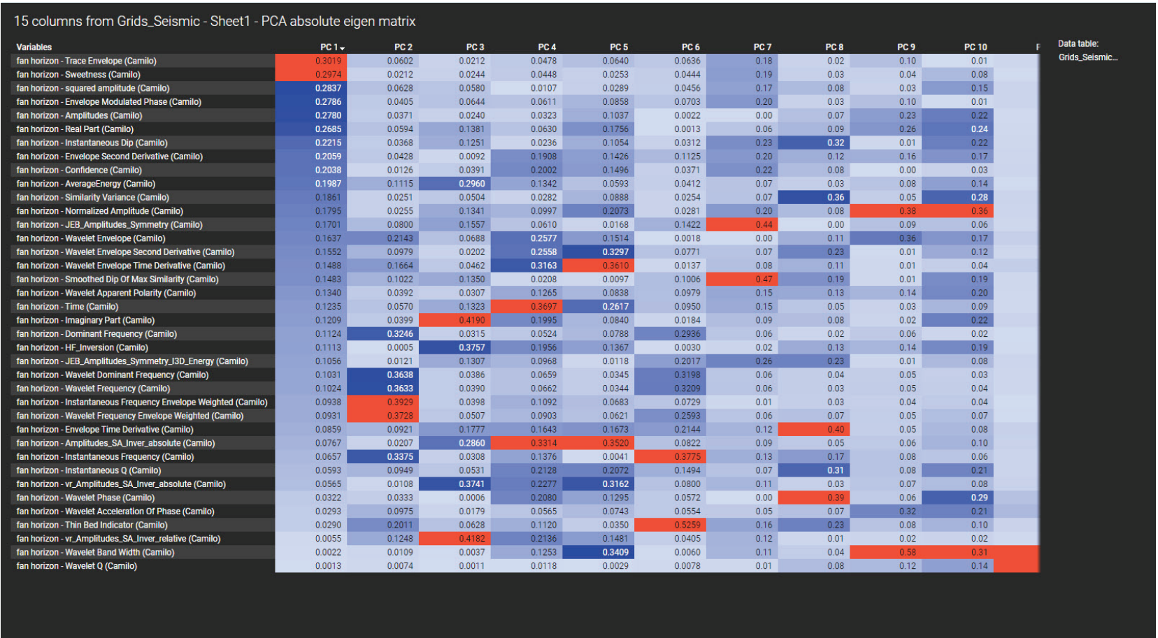
Figure 4: Analytics Explorer table results of PCA, indicating which input features are most represented at each principal component line. Interpreters can use this table to determine which input features are the most relevant and use those features in advanced clustering workflows. The attributes shaded in red are the top two most important attributes in a given principal component line.
